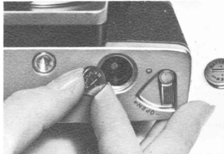
1. Remove the Battery Compartment Cover by turning it in the direction of the arrow with a coin.
