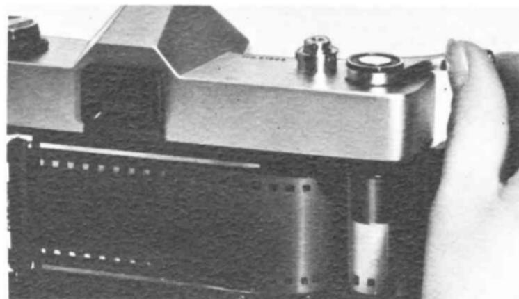
3. Insert the film leader into the Take-up Spool Slot and gently wind the film forward enough to wrap the end securely round the take-up spool. Make sure the sprocket teeth engage in the perforations in the film.
