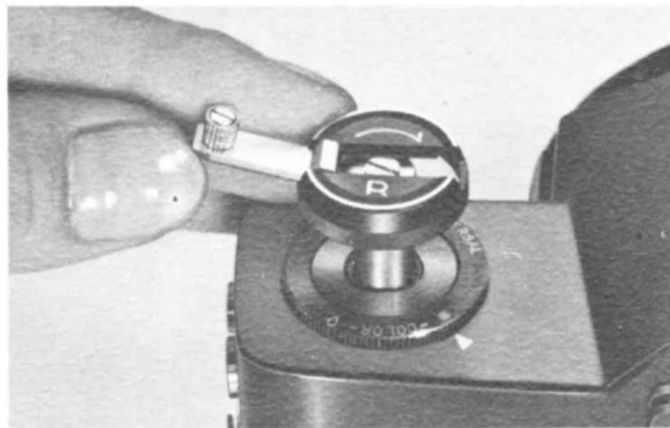
3. Fold out the Rewind Crank-Handle on the Film Rewind Knob and turn it in the direction of the arrow.
