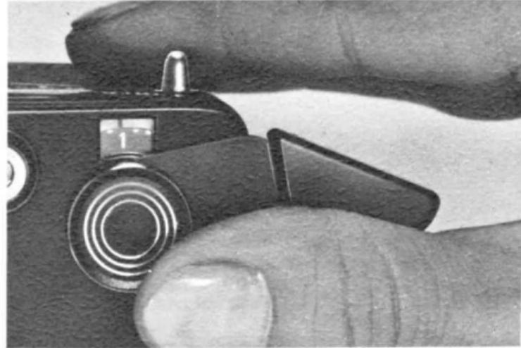
5. Advance the film by alternately operating the Film Advance Lever and depressing the Shutter Release Button until the Exposure Counter indicates the figure "1". You are then ready to shoot your first picture. The Exposure Counter shows you the number of the exposed frames.
